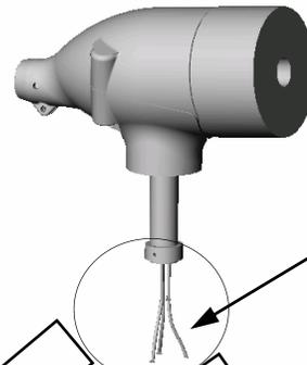
When the wires are unconnected the wind generator rotor should spin freely.
