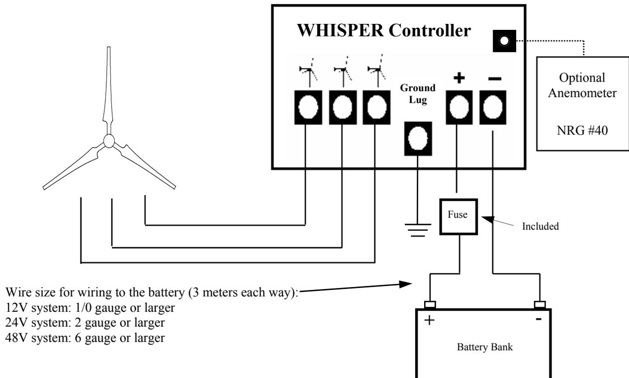
Once startup is successful and the red LED can be cycled by toggling the Diversion Switch, then set the switch to “Stop” (Red LED on) and connect the turbine wires to the controller (order of the turbine wires is not important). With the Red LED is on, the turbine will not spin as long as at least two of its wires are connected. For further operational information refer to Whisper Controller Operation on page 22.
