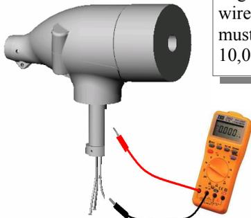
Check resistance to ground on any wire. Resistance must exceed 10,000 ohms.
